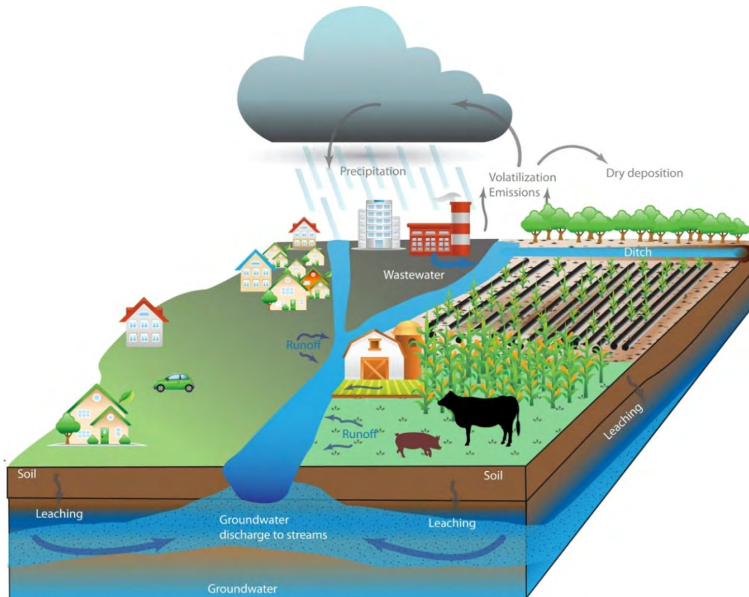
Figure 7. Nitrogen sources and pathways to streams, including direct discharges, runoff, leaching to groundwater, subsurface tile drainage to ditches, and precipitation directly into waters.
